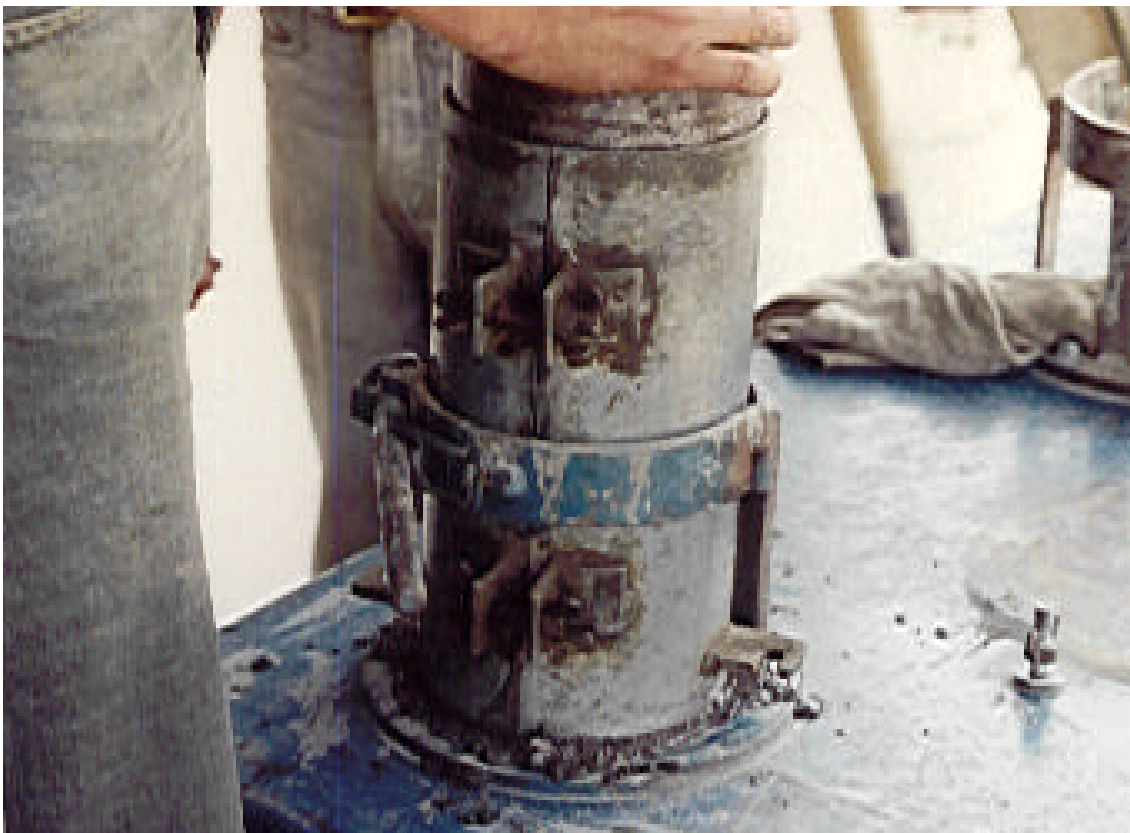
FIGURE 3- RCC Test Specimen Molding using the Vibrating Table.
