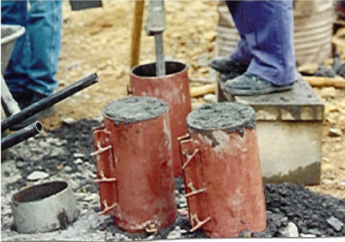
FIGURE 4- RCC test specimen molding using the pneumatic compactor
