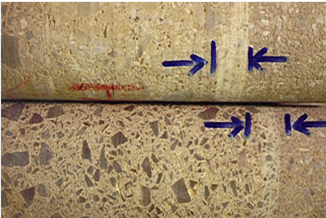
FIGURE 12-CORE DRILED FROM THE RCC TEST FILL, SHOWING THE ACTION OF THE BEDDING MIX PLACED ON THE CONSTRUCTION-JOINT OF CAPANDA DAM
