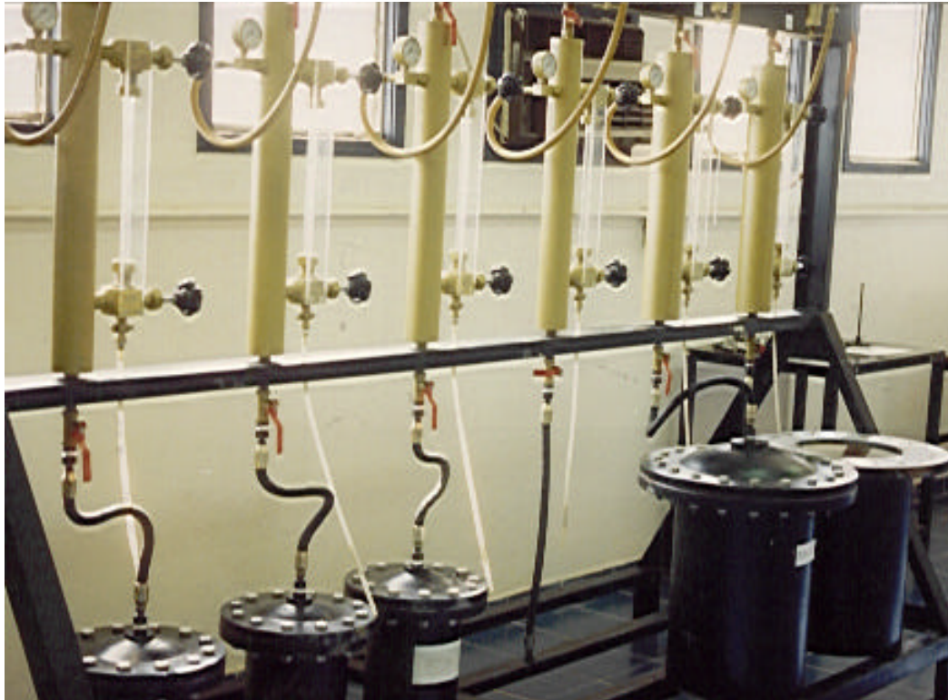
FIGURE- 23 -PERMEABILITY APPARATUS OS TEST, AT CAPANDA LABORATORY
