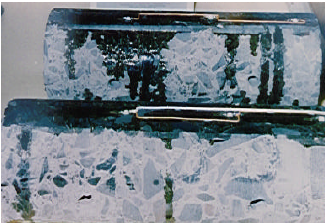
FIGURE 7- STRAIN GAGE USED OUTSIDE RCC DRILED CORE SPECIMENS FOR CREEP AND THERMAL EXPANSION TESTS.
