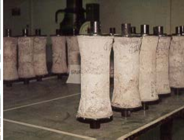
Photo 5. Horizontal joints specimens used to measure direct tensile strength.
