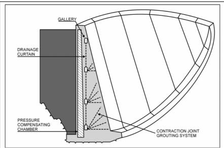
Figure 06- Andsar RCC Arch Dam- Galleries & PCC- Cross Section
