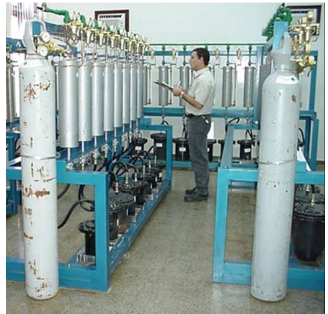
Figure- 31 -Permeability apparatus test, at FURNAS laboratory- Brazil
