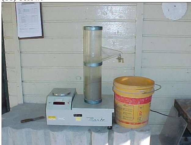
Figure 11- Device for determination of unit weight and unit water of RCC
