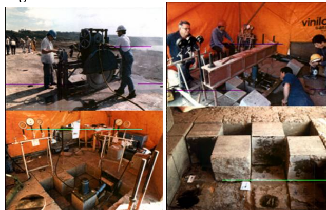
Figure 23- Biaxial shear test in situ at Salto Caxias Dam- Brazil
