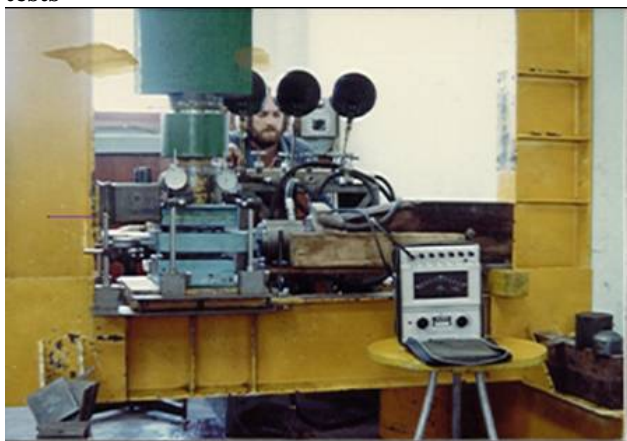
Figure 20- Biaxial shear test apparatus
