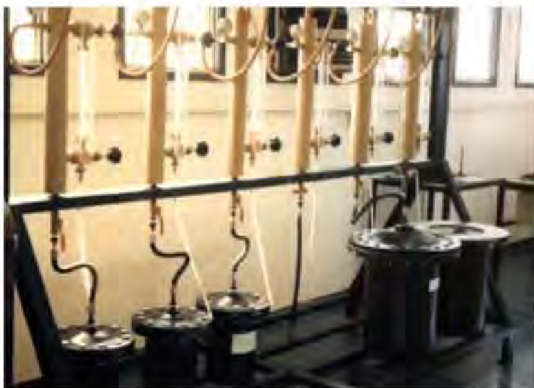
Figure 7.44 Permeability apparatus test at Capanda laboratory.
