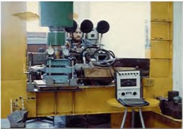
Figure 7.20 Modification in the apparatus shown in Figure 7.19, by changing the shear load angle, at Itaipu laboratory, as suggested by Bureau of Reclamation [7.56].
