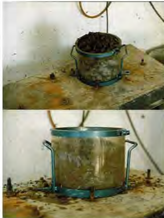
Figure 5.24 Consistency test of RCC mix using water-reducer /set retarder admixture.
