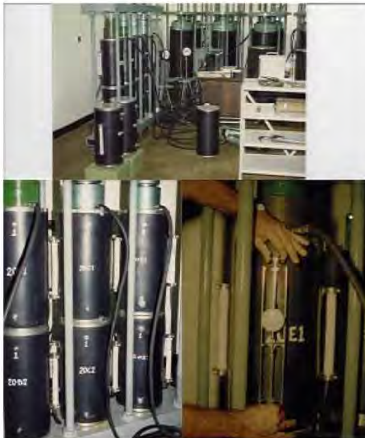
Figure 7.32 Capanda RCC and CVC specimens under a creep test, at Itaipu concrete laboratory.
