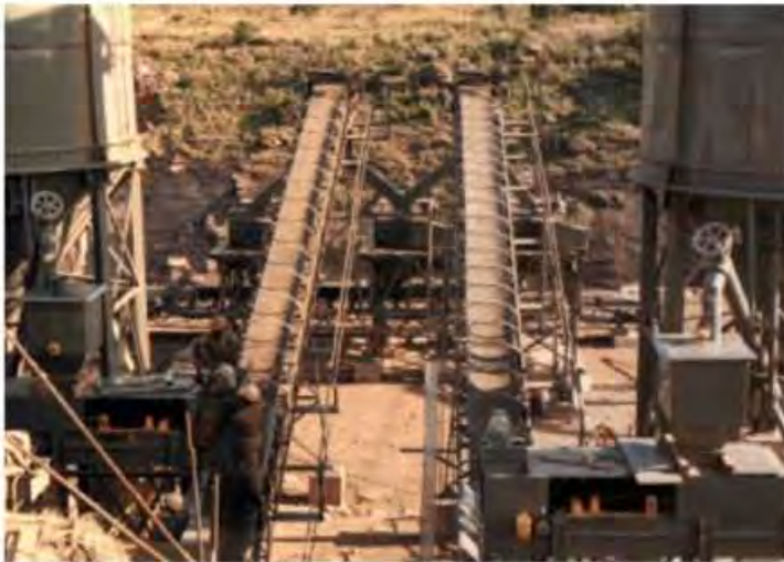
Figure 8.14 Continuous mixers used for RCC production, in Capanda dam-Angola.
