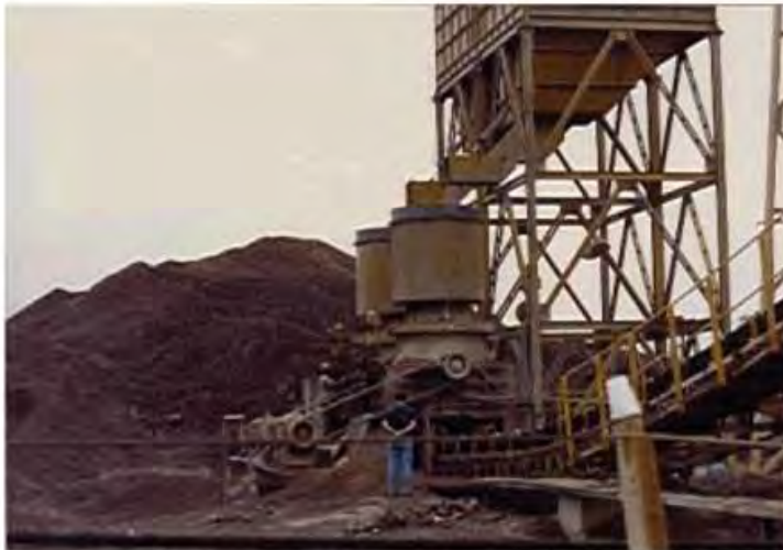
Figure 5.08 Hydrofine Recrushers at Capanda Dam site.
