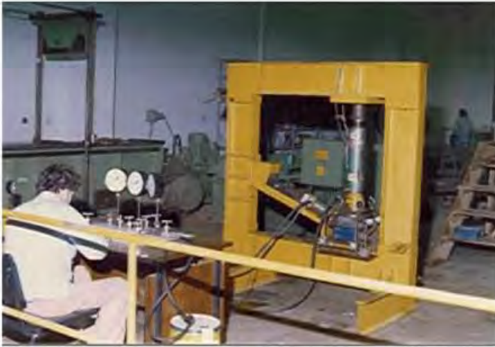
Figure 7.19 System used for biaxial shear test on rocks and concrete specimens, at Itaipu laboratory.
