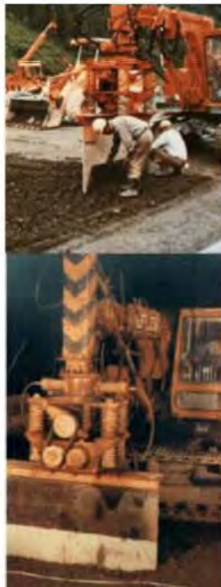
Figure 8.89 Joint cutter machine used at Japanese and Chinese dams.
