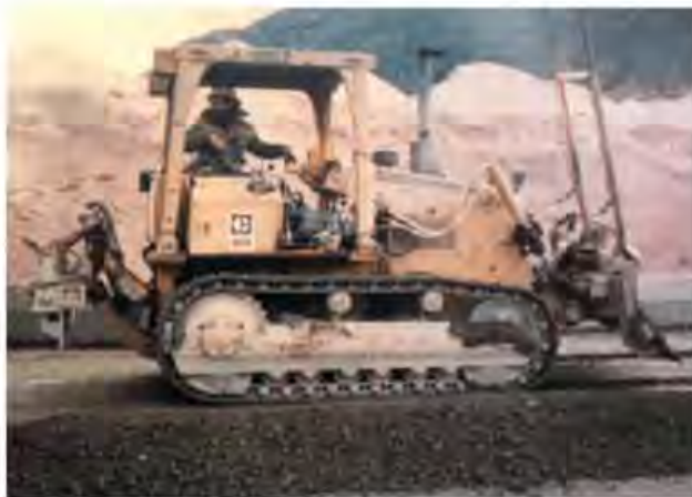
Figure 9.38 Laser sensor for grade control installed at dozer blade at Upper Stillwater dam - USA.
