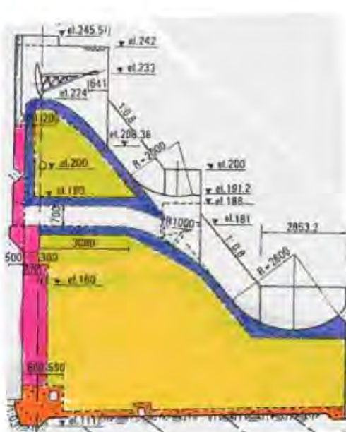
Figure 4.12 Concrete zoning diagram at Jiangya Dam (from [4.22]).
