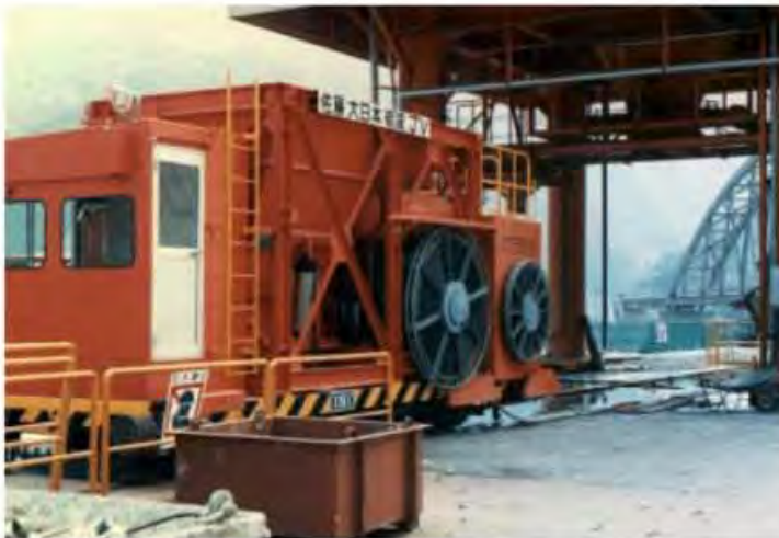
Figure 8.38 Hopper used to transport RCC, at Sakaigawa dam-Japan.
