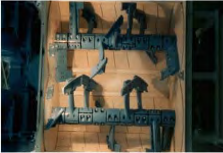
Figure 8.16 Batching twin shaft with two-axis paddle mixer used for RCC production, in the Japanese dams mainly.
