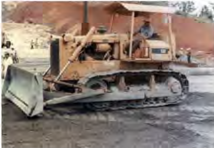
Figure 8.45 Dozer tracks provided with street pads to minimize damage to the compacted surface.
