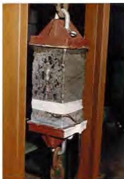
Figure 7.36 Tensile strain tests – Close view showing the wire strain gage on RCC specimen surface.
