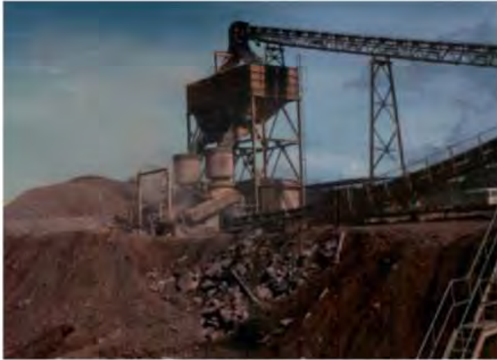
Figure 8.10 Crushers to produce crushed sand and powder filler near the batching plant, at Capanda dam-Angola.
