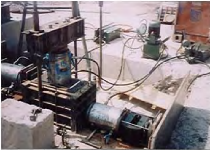
Figure 7.25 Biaxial shear - in situ - test undertaken at Capanda test-fill.
