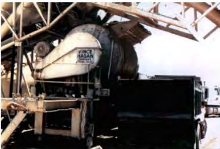
Figure 8.17 Batching ribbon mixer type for RCC production, for pavements mainly.
