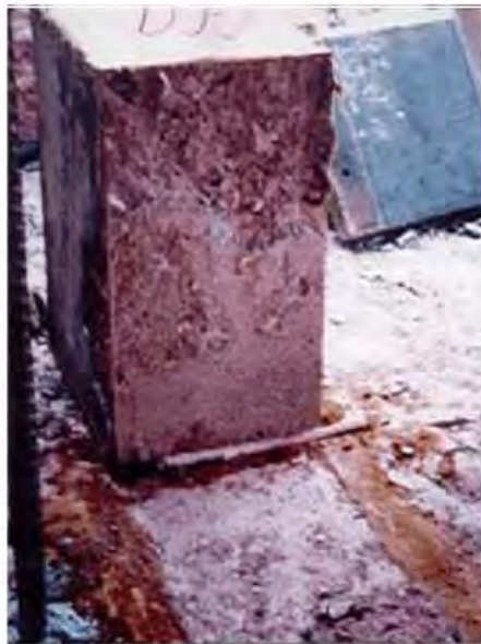
Figure 7.27 RCC blocks specimens after tested, showing that the bedding mix works well and the failure surface occurred immediately below the construction joint.
