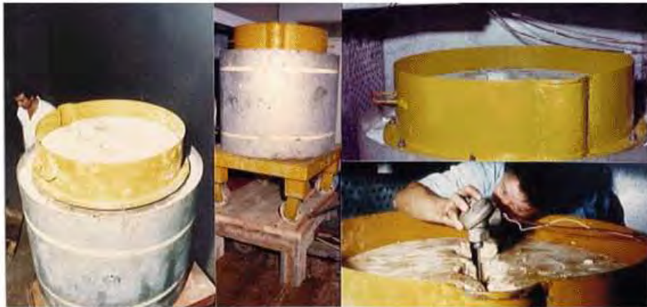
Figure 7.39 Adiabatic temperature rise test - Specimen inside the adiabatic room.
