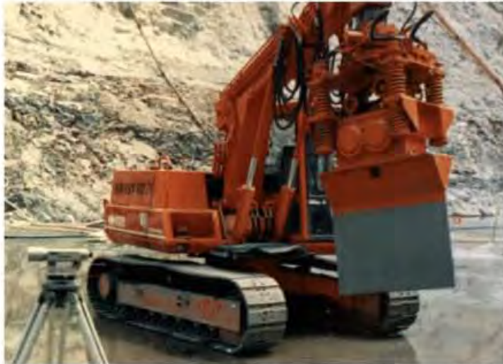
Figure 8.88 Back-hoe joint cutter machine used at Sakaigawa dam-Japan.
