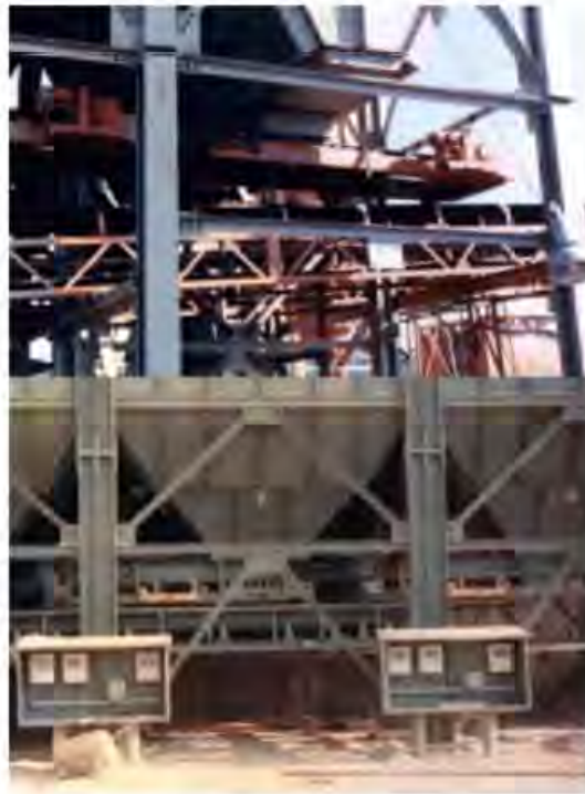
Figure 9.12 Load cells under the belt conveyor to provide weight control.
