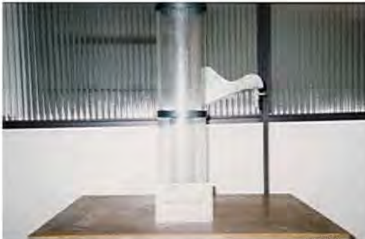
Figure 7.05 Device to determine unit weight and unit water of RCC.
