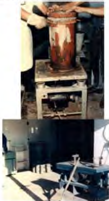
Figure 9.21 Vibrating Table being used for Cylinder Preparation-Itaipu Laboratory-1976 [9.19].
