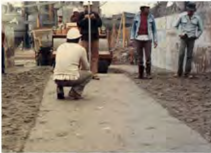
Figure 8.49 Tests being performed in test fills prior to early construction stages to determine the minimum number of passes required for full compaction, based on design mixture and topographic survey.
