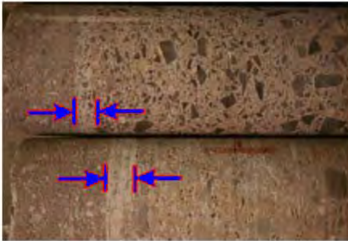
Figure 7.26 Core drilled from the RCC test-fill, showing the action of the bedding mix placed on the construction joint of Capanda dam.
