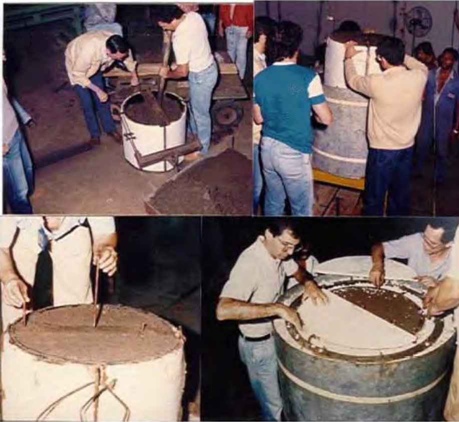
Figure 7.38 Adiabatic temperature rise test - Specimen preparation.
