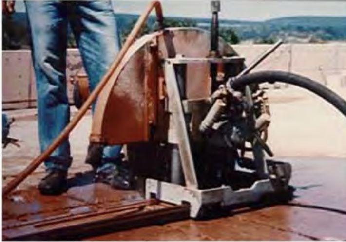
Figure 7.24 RCC block-specimens being cut by diamond saw blade, at Capanda job site.
