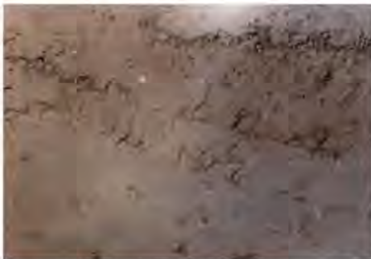
Figure 8.51 Over-compaction promotes a lamination on the RCC surface and may lead to lower densities and, thus, should be avoided. The top of a lift may become less dense while the bottom becomes denser.
