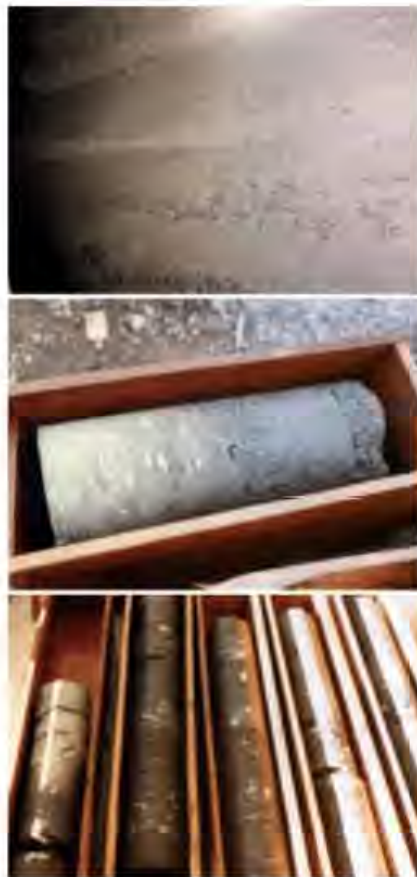
Figure 12.03 Segregation of coarse aggregate between lifts endeavoring lack of continuity
