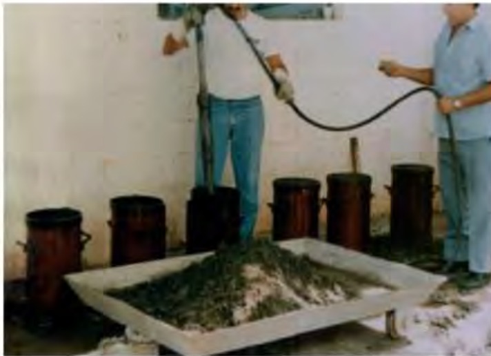
Figure 9.23 Pneumatic hand hammer being used for Cylinder Preparation-CESP Laboratory- 1993 [9.20].
