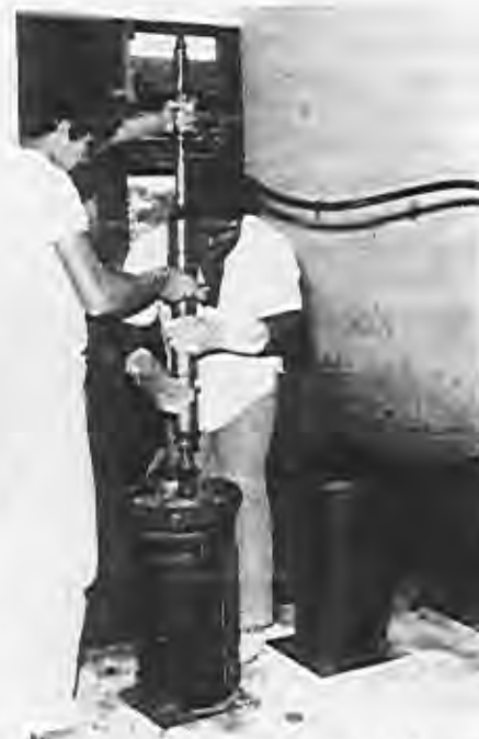
The molding of a cylindrical specimen and compacting with hammer tamper.
