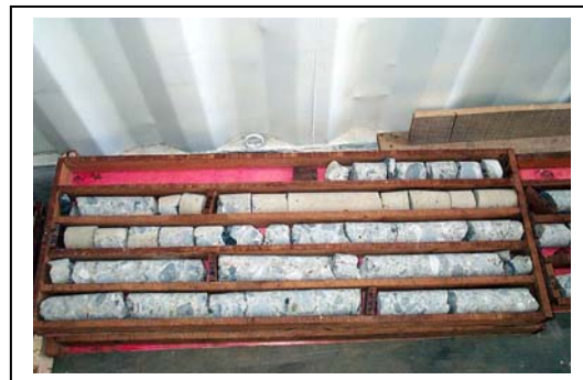
Figure 22- Drilled cores from diaphragm mortar, interface, and from the old concrete from the dam
