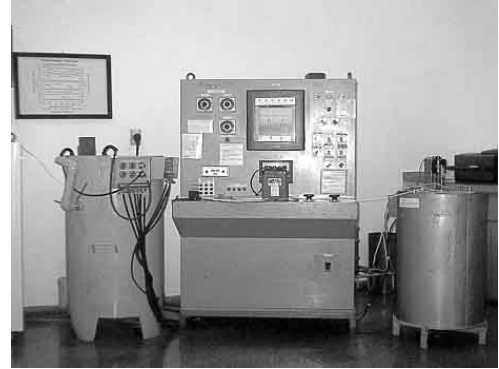
Figure 2.1 – Equipment for the Thermal Characterization of Concrete
