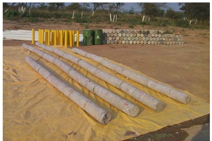
Picture 4 –Core drilled from the RCC
