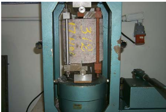
Picture 5 - Core of RCC - Direct Shear Test
