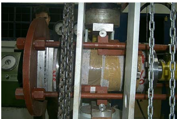
Picture 6 - Test core of RCC – Biaxial Shear Test.
