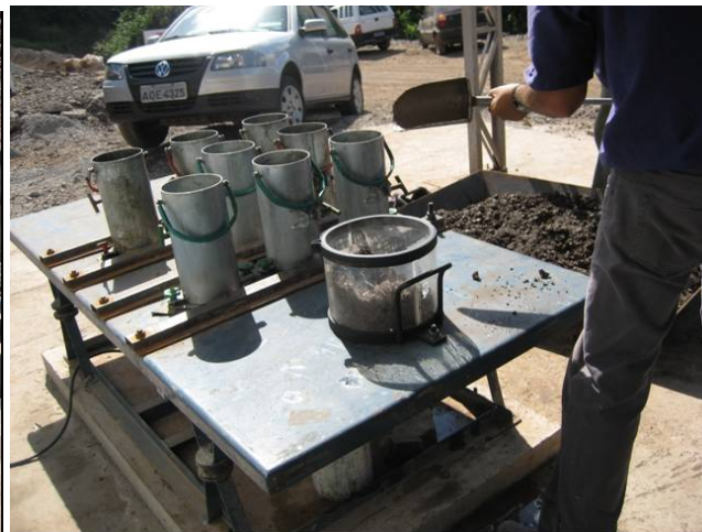
Figures E-53- Vibratory table for Consistency Test and for Cylinders Specimen
