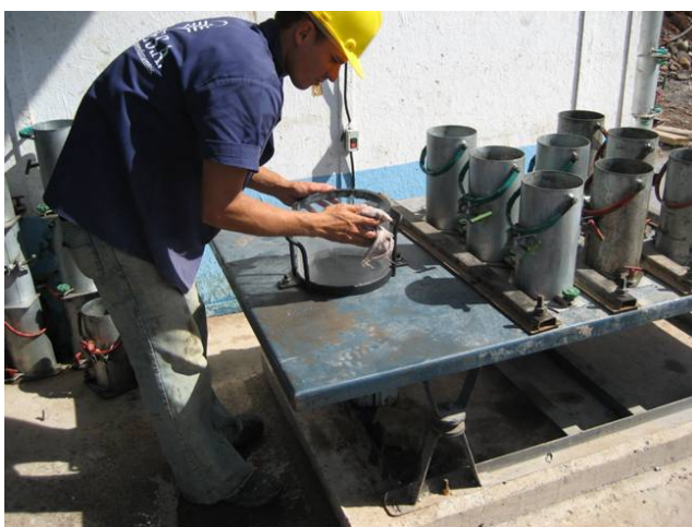
Figures E-53- Vibratory table for Consistency Test and for Cylinders Specimen
