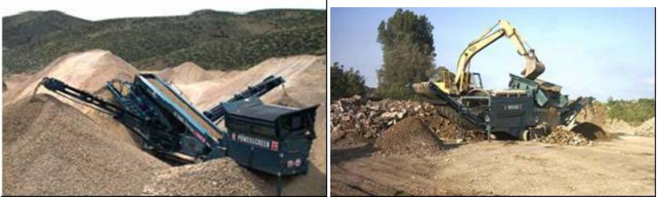
Figures E-14- Mobile equipment (Power Screen) suitable to classify aggregates from the alluvial deposits.
