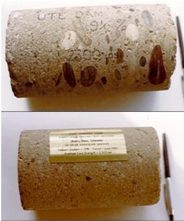
Figure 05- Soil Cement used as embankment protection in dams in the United States-Resistance greater than 17 MPa
