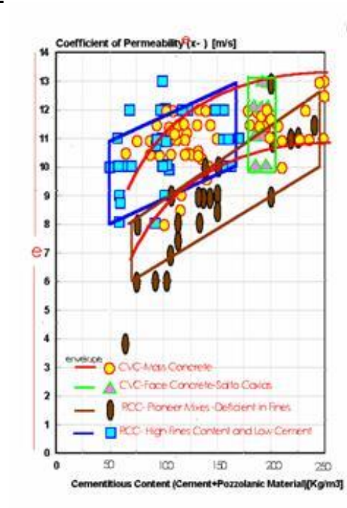
Figure 08– Permeability Results of Mass CVC and RCC. [23]
