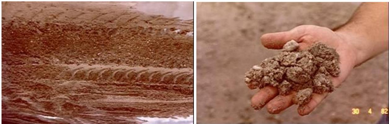
Figures 02- Aspects of Sandy Material for potential use for Soil-Cement 1982
